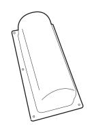
**1.** From inside hood of bin, remove FireSafe cover by unscrewing all six fixings with a screwdriver.
