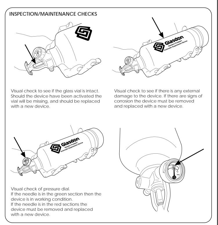
Glasdon FireSafe<sup>™</sup> is an effective low cost auxiliary device designed to quickly extinguish fire at source but is not intended to replace primary fire prevention measures. A regular inspection and maintenance programme will ensure the device is kept in good working order. In the event that the device has been discharged it must be replaced.
