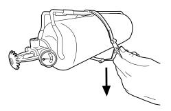
2. Release clasp on fixing bracket.
